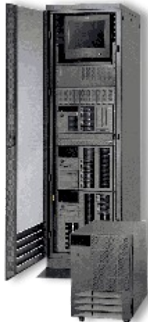
Rack Mounted Server
